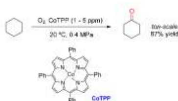
Scheme 1: First industrial-scale bioinspired oxidation of cyclohexane with CoTPP.
