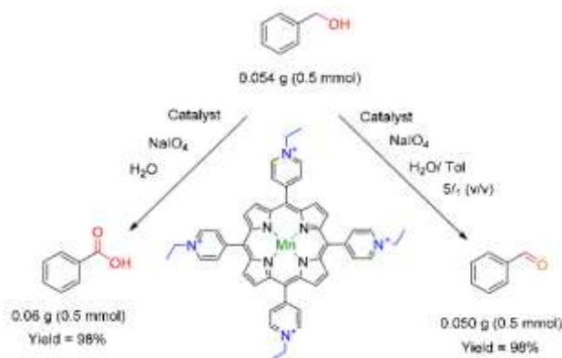
Scheme 7: Oxidation of benzylic alcohols to carbonyl compounds with a Mn-porphyrin.
